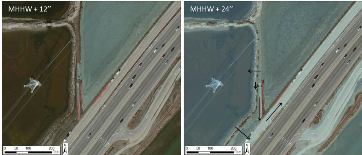
Figure 6. Effect of the sheet pile/concrete barrier and cross berm on inundation pathways in the MHHW + 12'' and 24'' scenarios.
