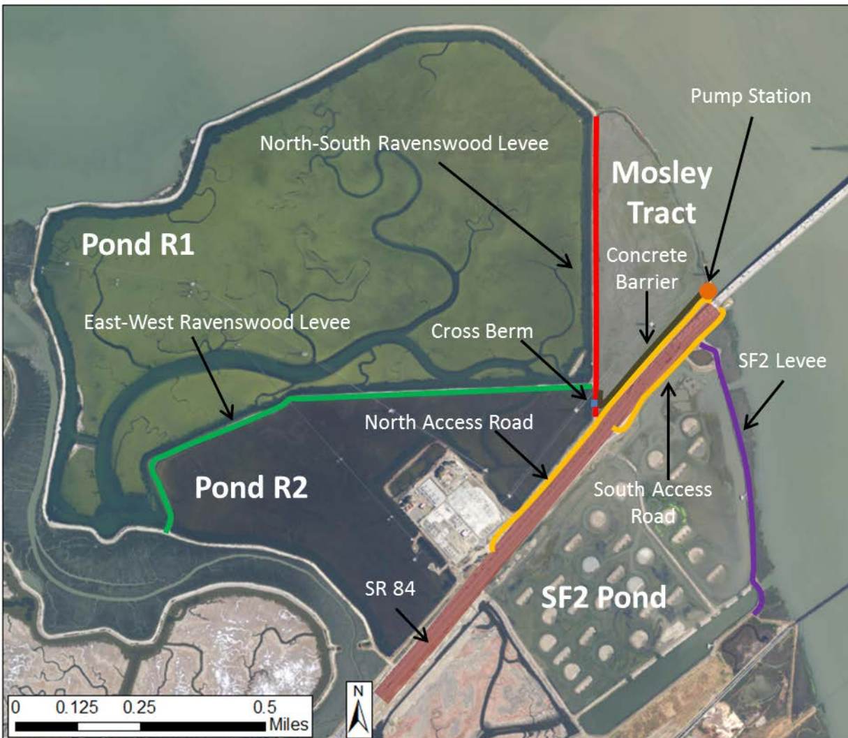
Figure 1. Focus study area showing ponds, levees, and recent temporary flood construction
