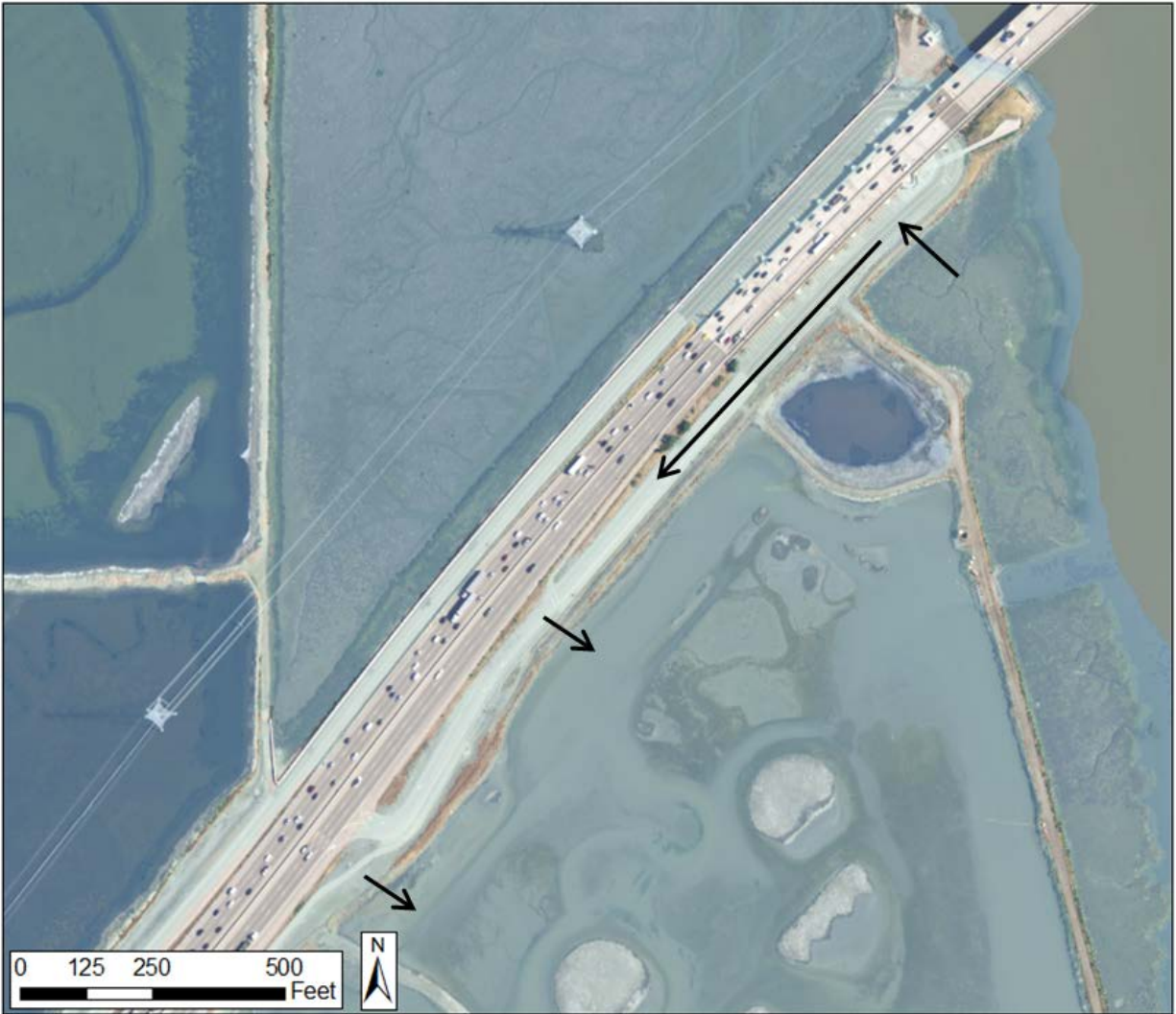
Figure 3. Inundation of area south of SR 84 in MHHW + 24'' scenario. Arrows indicate the inundation pathway.
