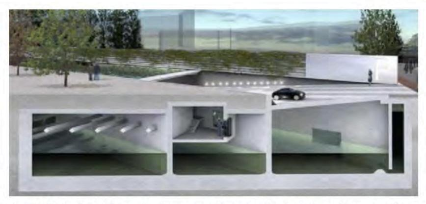
Figure 4. Multi-functional underground parking garage used as a reservoir for floodwaters and storm waters (Aerts et al., 2009).
