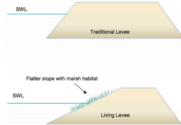
Figure 6-4: Conceptual diagrams of a traditional levee (top) and living levee (bottom)
