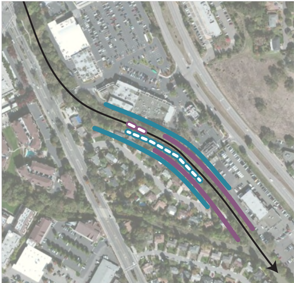
Figure 3.15. Novato Creek HOT Summary. This plan view shows the results of the desktop and field investigations for both the current and future HoT zones. Compared to other sites, the future zone will not migrate far upstream, most likely because of the steep slope of the channel at the current HoT.
