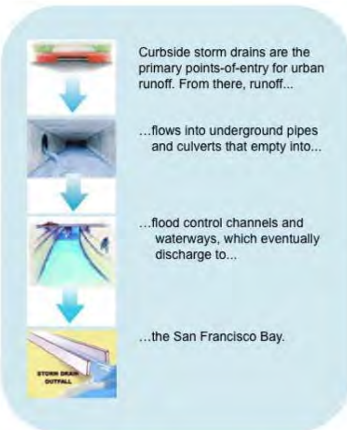
Figure 1. Overview of urban stormwater infrastructure, from curb to Bay. Source: Adapted from www.lastormwater.org/siteorg/general/lastormdrn.htm
