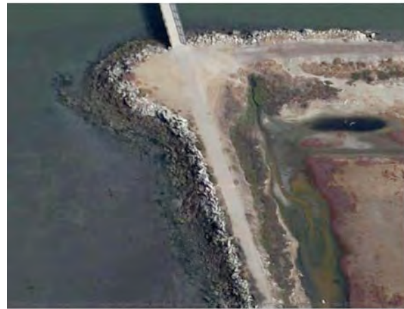
Figure 4. Non-engineered berm with riprap on outboard side (Source: Google Earth).
