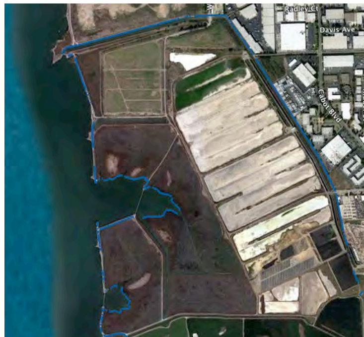
Figure 15. With 16 inches of sea level rise, 30% of system #23 will overtop with an average depth of 2 feet during a storm event (areas shown in blue). The overtopping is mostly along Depot Road adjacent to industrial and commercial businesses.
