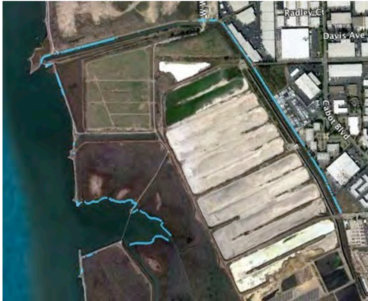
Figure 16. With 55 inches of sea level rise, almost 70% of system #23 will overtop with an average depth of 2 feet (area in dark blue). The majority of overtopping will occur along Sulphur Creek and Depot Road levees, and along the Bayshore non-engineered earth berms.
