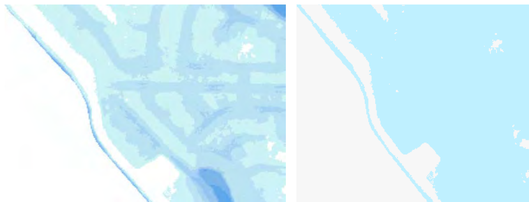
Figure 2 Comparison of flood depth layer (left) with binary flood layer (right).
