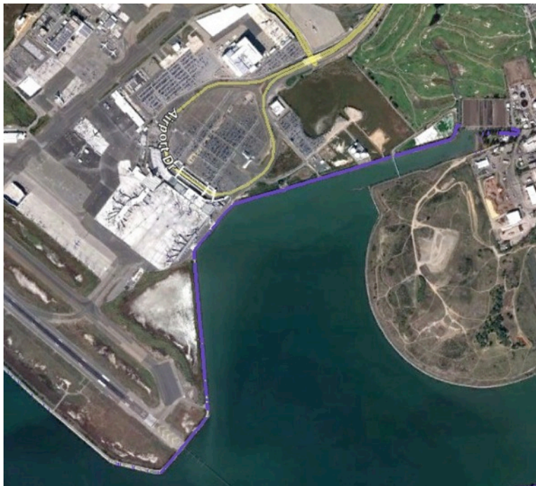
Figure 13. The northern portion of Bay Farm Island, from the Bay Farm Island Bridge to Aughinbaugh Way, is protected by a non-engineered earth berm structure, and is vulnerable storm events with sea level rise.
