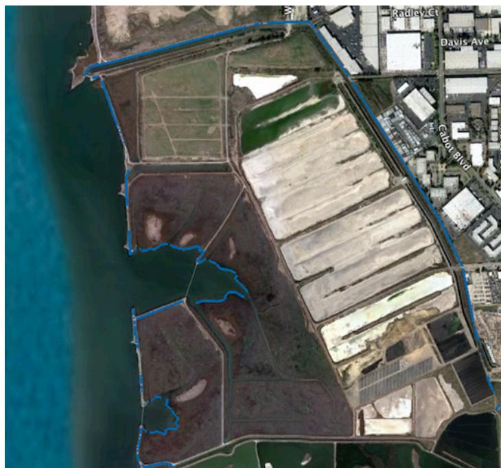
Figure 15. With 16 inches of sea level rise, 30% of system #23 will overtop with an average depth of 2 feet during a storm event (areas shown in blue). The overtopping is mostly along Depot Road adjacent to industrial and commercial businesses.
