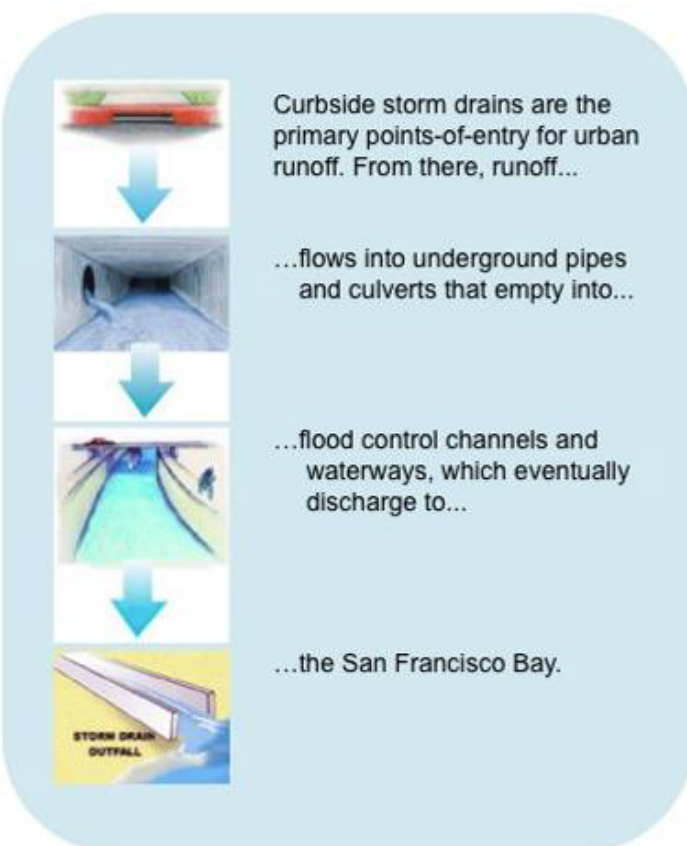
Figure 1. Overview of urban stormwater infrastructure, from curb to Bay. Source: Adapted from www.lastormwater.org/siteorg/general/lastormdm.htm
