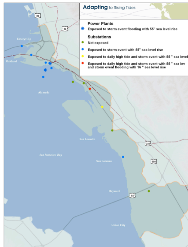
Figure 2. Exposure of power plants and substations to daily high tide and storm events with 16 and 55 inches of sea level rise
