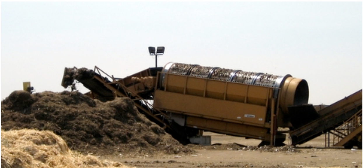
Compost screener at work. Source: http://www.ethicurean.com/2008/07/14/food-scrap-composting/ .
