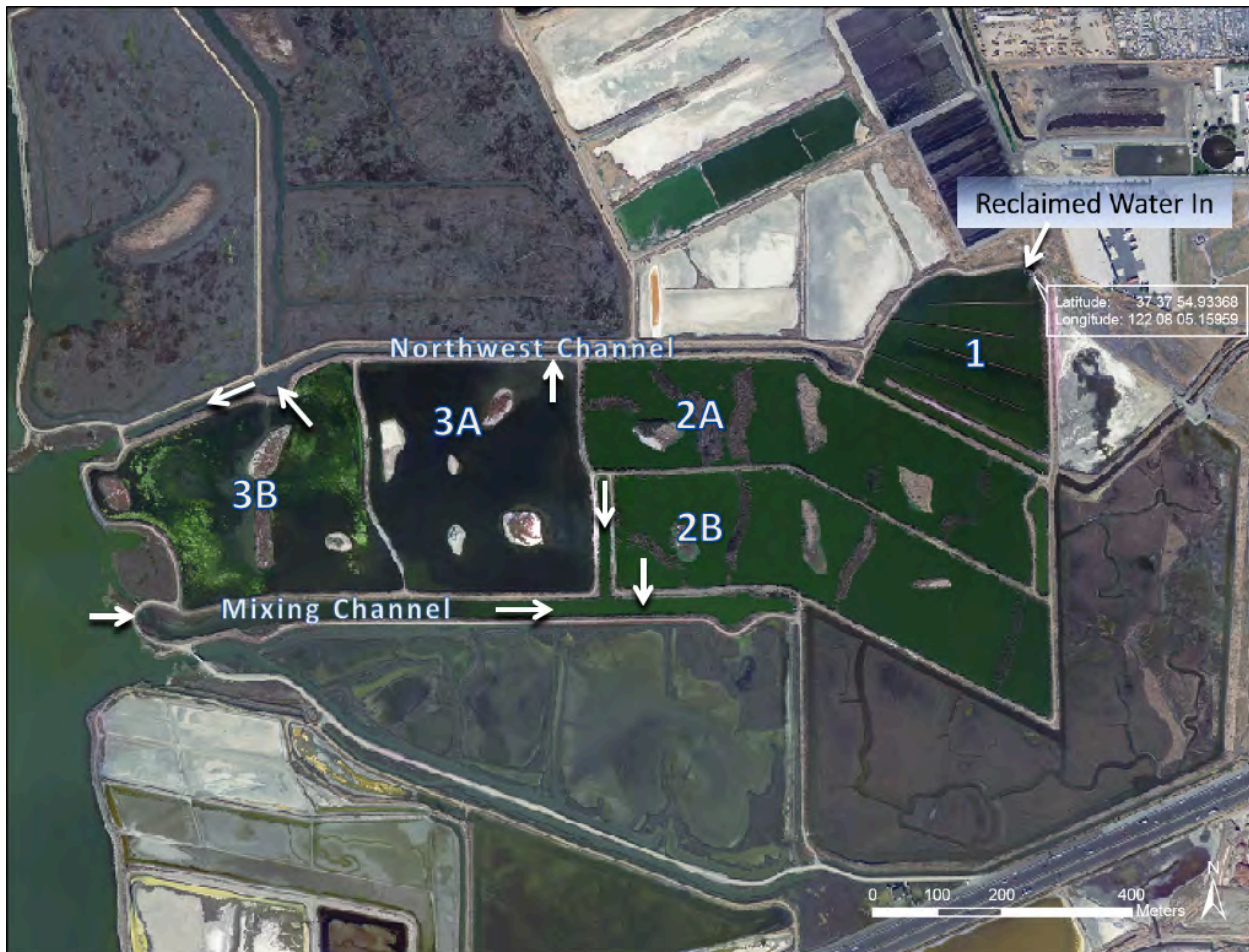
Map of Hayward Marsh showing specific ponds and channels under investigation (prepared by RMC Water and Environment as part of Hayward Marsh Rehabilitation Options Study). Basins 1, 2A, and 2B are freshwater ponds, while basins 3A and 3B are brackish ponds. Tidal waters are designed to mix in Basins 3A and 3B, but not Basins 1, 2A, and 2B. The outboard levee along basin 3B is part of the Bay Trail.
