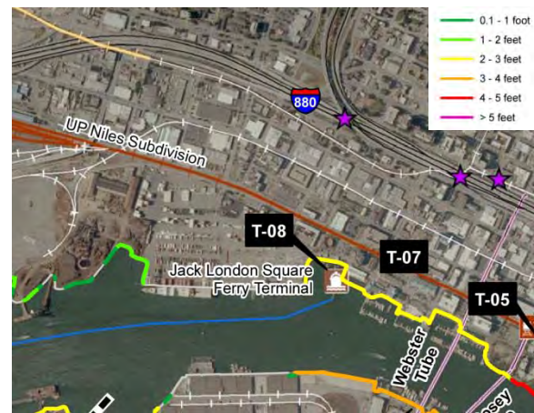
Projected Overtopping Depth at 55 inch SLR + 100-yr SWEL
