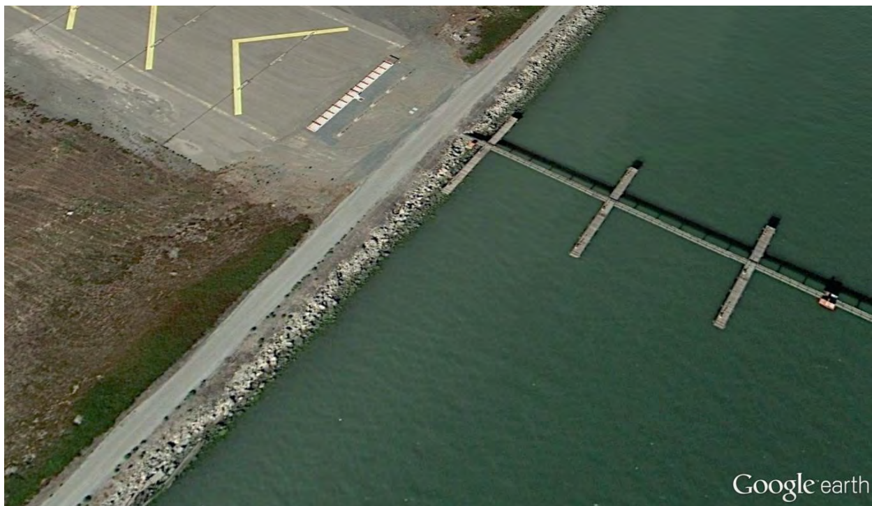
Figure 2.4 Engineered Levee with Revetment: Oakland International Airport, Oakland; Roadway Is Levee Crest
