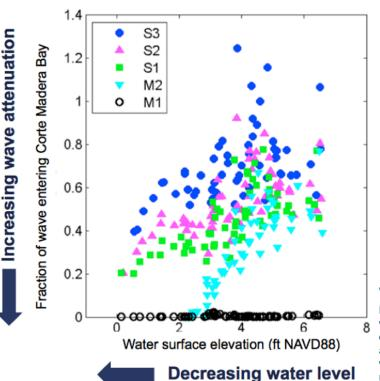
dramatically from the mudflat to the marsh. Wave attenuation is largely determined by water depth, therefore wave height and energy are significantly reduced at the marsh edge. Vegetation on the marsh plain provides additional wave attenuation, regardless of species (i.e., cordgrass or pickleweed). Marsh downshifting due to sea level rise will increase water depths and decrease wave attenuation, and a wider marsh will be needed to maintain flood risk reduction benefits.
